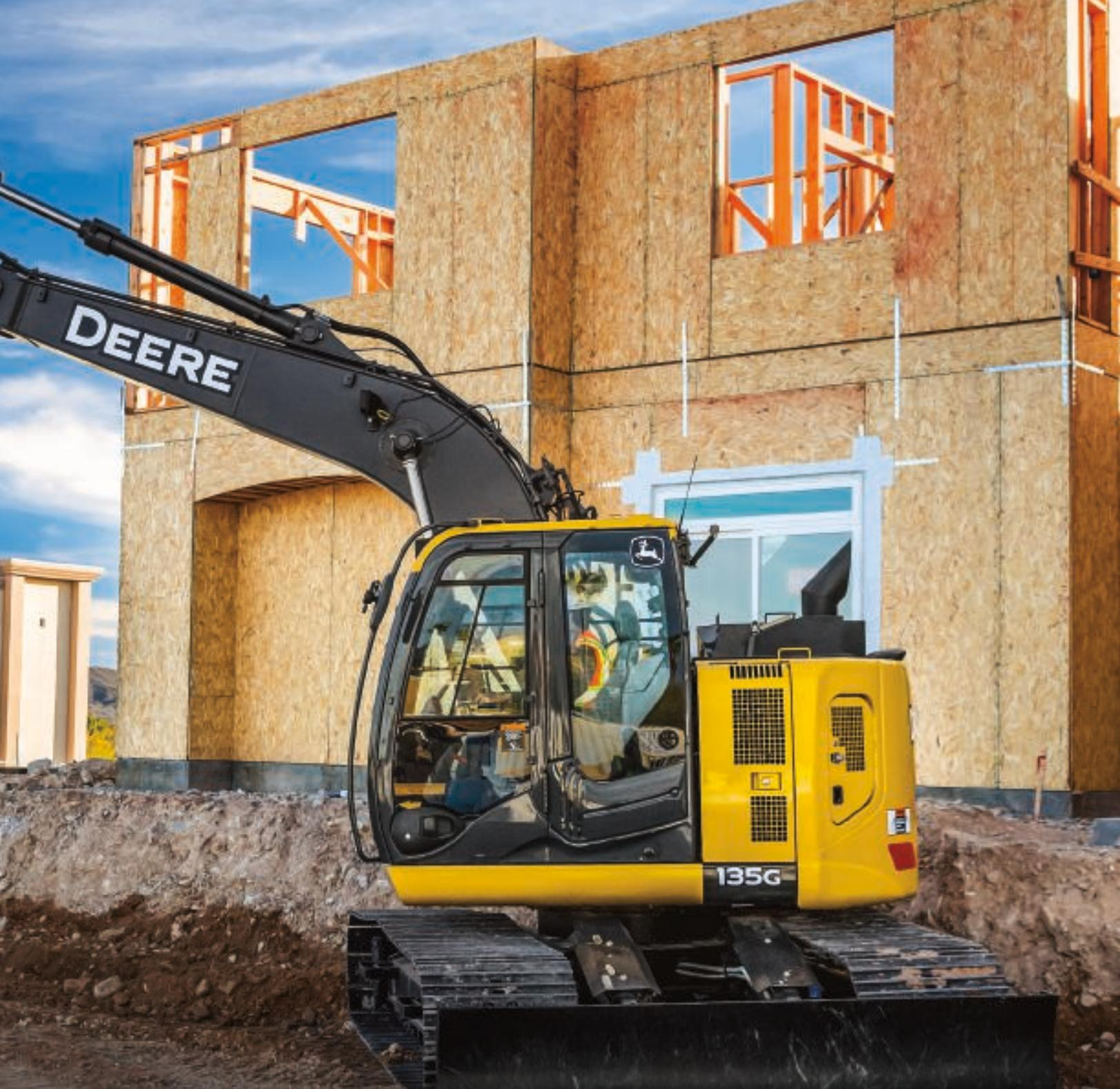
1. With large idlers, rollers, and strutted links, the sealed and lubricated undercarriage delivers long and reliable performance.
