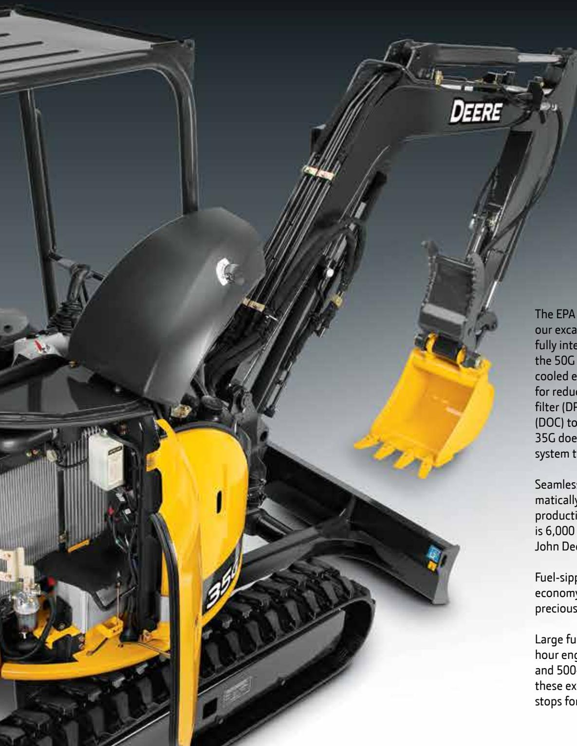
The EPA FT4/EU Stage IV technology in our excavators is simple, fuel efficient, fully integrated, and fully supported. In the 50G and 60G, it employs field-proven cooled exhaust gas recirculation (EGR) for reducing NO<sub>x</sub>, and a diesel particulate filter (DPF) and diesel oxidation catalyst (DOC) to reduce particulate matter. The 35G doesn't require an after-treatment system to meet EPA requirements.
