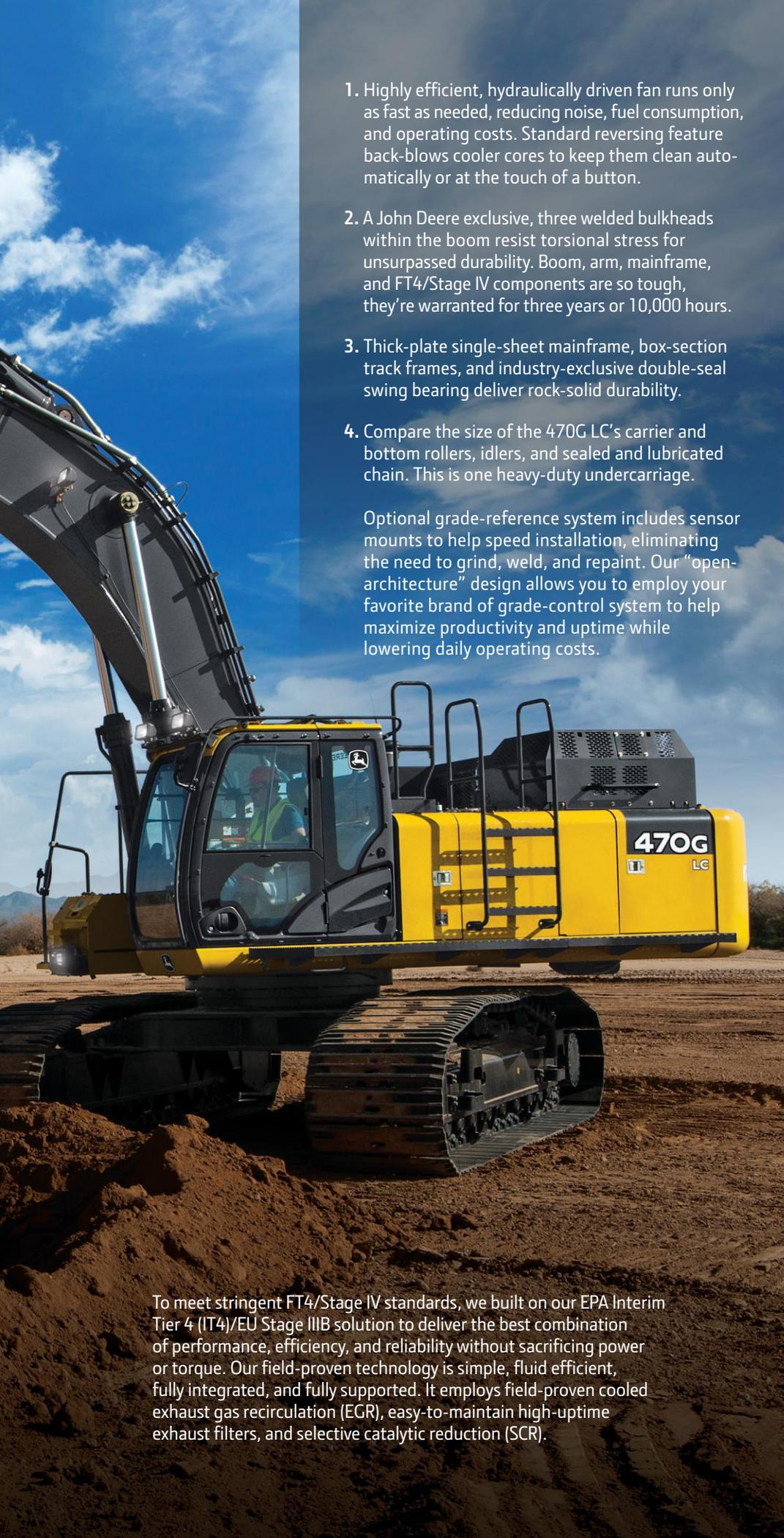
1. Highly efficient, hydraulically driven fan runs only as fast as needed, reducing noise, fuel consumption, and operating costs. Standard reversing feature back-blows cooler cores to keep them clean automatically or at the touch of a button.
